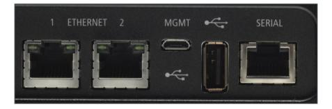
The Aprisa SR+ provides four data ports, buildconfigurable to have 2, 3 or 4 Ethernet ports on a single radio with the remainder as RS-232; ultimate flexibility for migration and connected devices.
