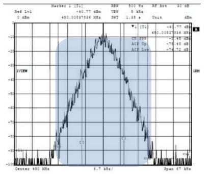
Aprisa SR and other radios use the robust FSK modulation, using little over half of the available spectrum. The Aprisa SR+ with new technology offers QAM modulation, using the full spectrum and delivering up to 5 times more capacity.
