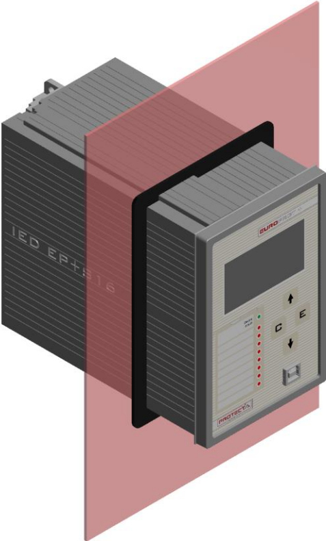
Figure 4-3: S16 semi-flush mounting method (max. depth = 75mm)
