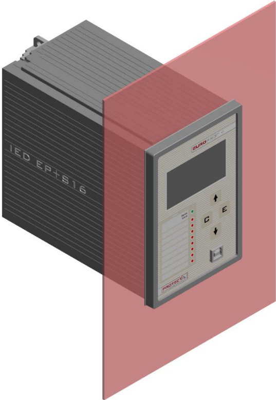
Figure 4-4: S16 flush mounting method
