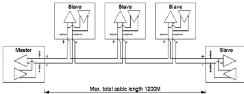
The topology of an RS-485 network using Kamstrup isolated and failsafe RS-485 slave or add-on modules.
